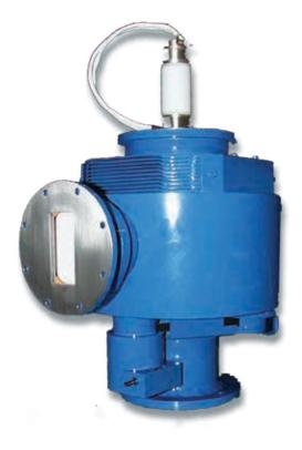
A magnetron is a high power microwave oscillator in which the potential energy of an electron cloud near the cathode is converted into RF energy in a series of cavity resonators. The VMS1197B magnetron delivers high peak and average RF power for use in medical or industrial applications.
